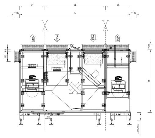
SUP operating side to the left or right as required, also connectors (SUP, EHA) at the top or front
